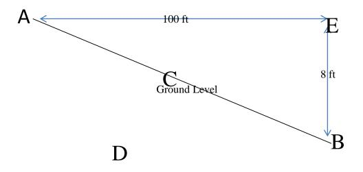
Flags are 100 feet apart (A and B). From the approximate center of the 100 feet(C), step about 15 steps toward to the low side of the slope. (D)With a straight edge or using your arm extended at the ground level of (A), swing your body keeping straight edge or your arm level, locating point (E) directly above flag (B). The measurement of (E) to the ground is percent or foot of fall in elevation from (A) to (B).
