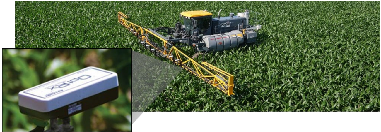
Figure 1: Active crop canopy sensor (left) positioned over the corn canopy and high-clearance applicator (right) equipped with OptRx® crop canopy sensors, GPS, and drop nozzles.
