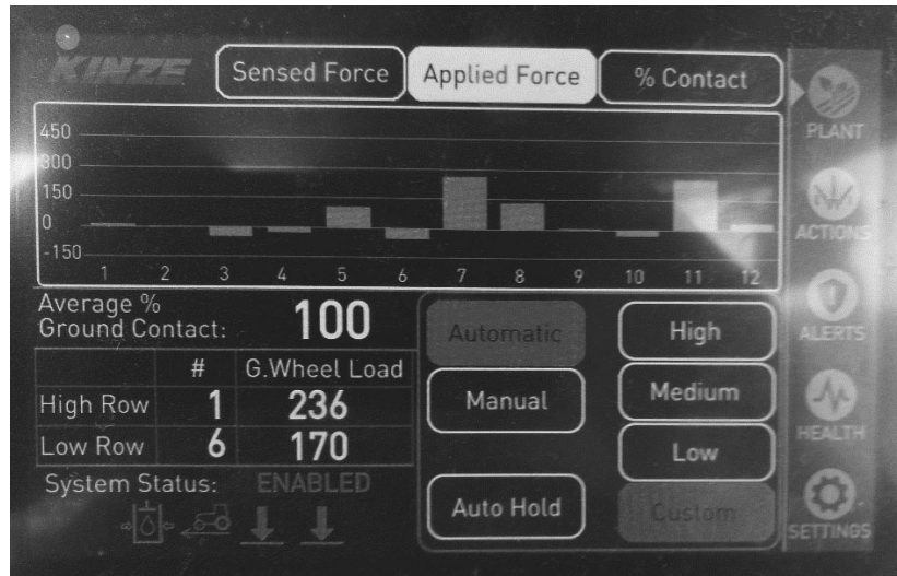
Figure 2. Image of monitor showing the applied force with the automatic down pressure set at 180 lb total downforce.
